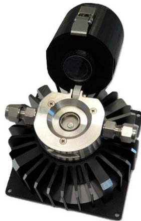
Figure 3: Dewtran II sensor open
